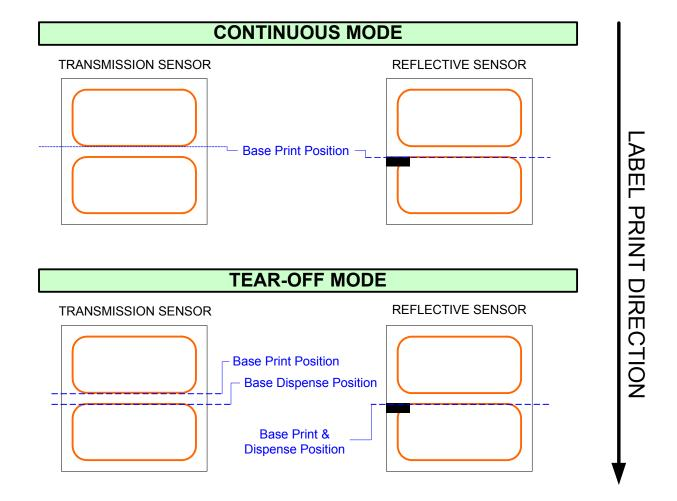
Figure 7-2, Label Reference Position Diagram
